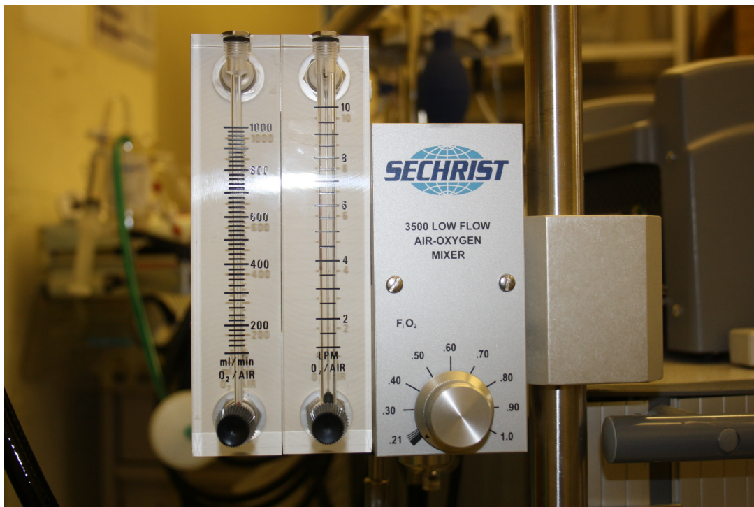
Figure 8 Type: High/Low flow Oxygen flowmeter & Air/Oxygen blender
